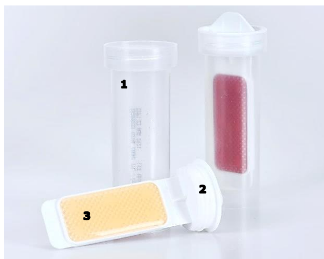
Figure 1. Components of HygieneChek™ PLUS dip-slides (1 – tube-container; 2 – screwcap-slide; 3 – agar)
